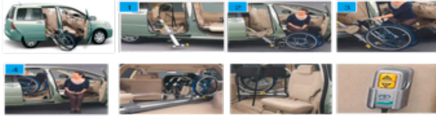
b) Toyota manual-wheelchair electro-motion wheelchair keeping device
